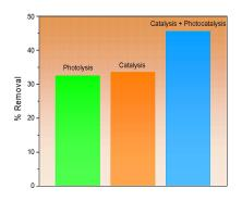
The catalyst was able to remove 33.5% of PCT upon 6h of agitation at room temperature ( $24^{\circ}C$ ) without irradiation, compared to 32.4% of removal of PCT from solution upon 6h of UV-VIS irradiation. Irradiation of the PCT/catalyst solution/suspension for 6h yielded 44.5\% removal of PCT, thus showing that the catalyst also has photocatalytical activity in the removal of paracetamol from an aqueous solution.
