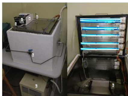
Figure 1: UV-C light chamber irradiation: 1) temperature display (Digimec – BTC 9090); 2) Microprocess (TT-34); 3) adjustors; 4) Termocouple-j; 5) Valve control (Hoke); 6) Thermobath; 7) UV-C-lamp ; 8) Cooler (Intel).
